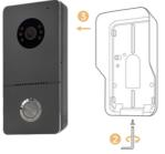
4. Pass the 4-core wire through the hole in the wall.
